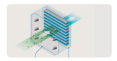
The PM1.0 filter is not only effective at capturing ultrafine dust up to  $0.3\mu m$  in size, but it also sterilizes up to 99% bacteria.
